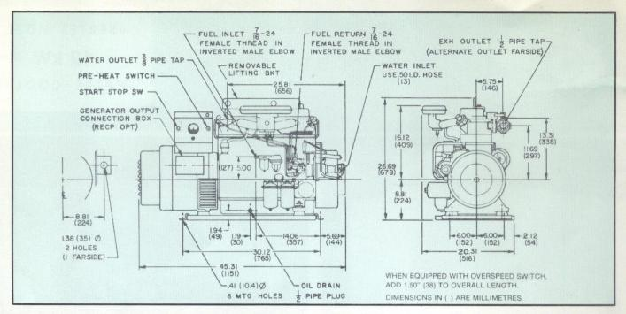
Add approx 1-in (25.4 mm) to overall dimensions for Heat Exchanger Cooled Models. Approx net weights: Raw Water Cooled 745-lb (337.93 kg). Heater Exchanger Cooled 765-lb (346.90 kg). Operation
